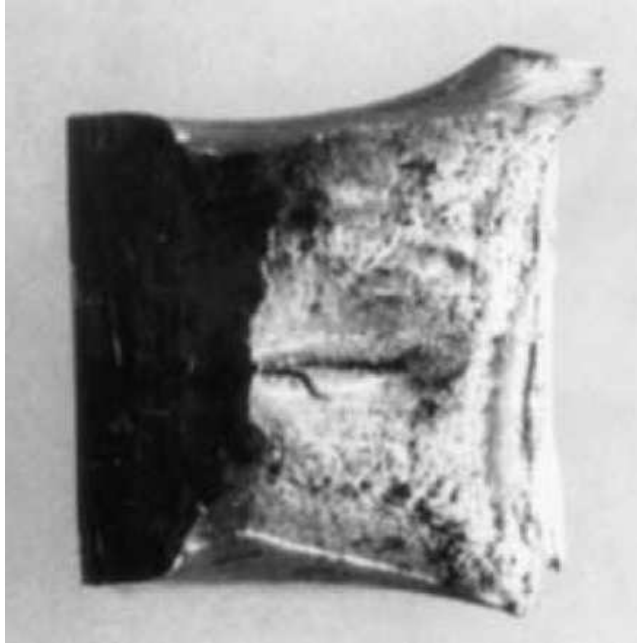
Figure 8: The feature normal to the length of the Charpy notch is a ‘split’ which influences the impact energy measured. Reproduced with permission of Elsevier from [63].
