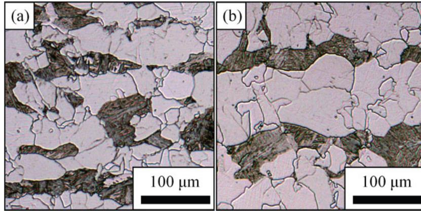
2 Optical micrographs of a Ti-Nb and b Ti-Nb-Mo steels after isothermal treatment at 700°C for 40 min
