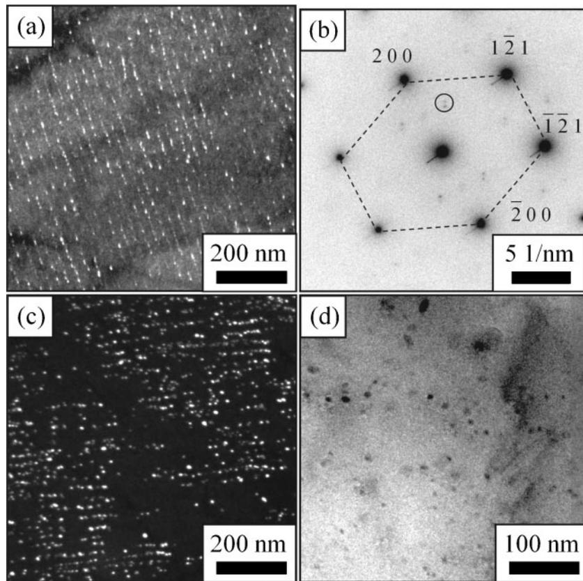
a dark field image after isothermal treatment at 700°C for 40 min and b its corresponding diffraction pattern; c dark field image after prolonged aging at 650°C for 24 h; d carbon replication image after prolonged aging at 700°C for 120 h
