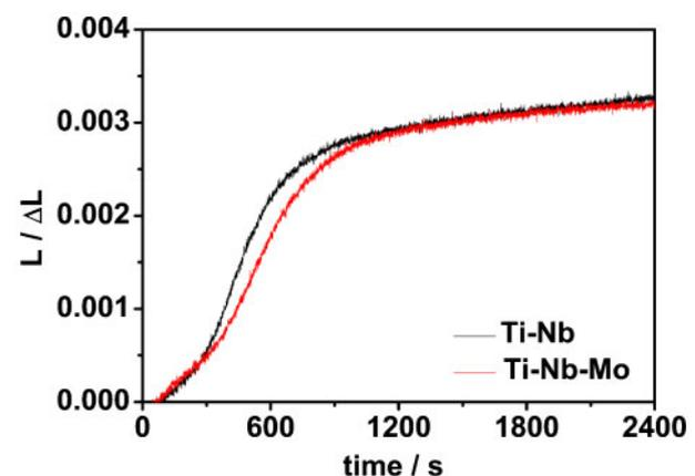
**5 Dilatation curves of Ti–Nb and Ti–Nb–Mo steels during isothermal treatment at 700°C for 40 min**
