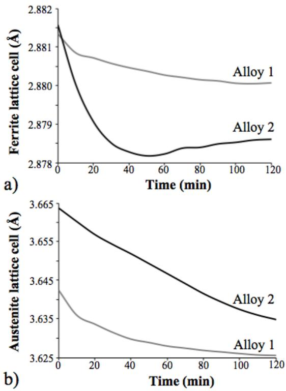
Fig. 4. Lattice parameter changes of (a) bainitic ferrite and (b) retained austenite during isothermal tempering at 520°C.
