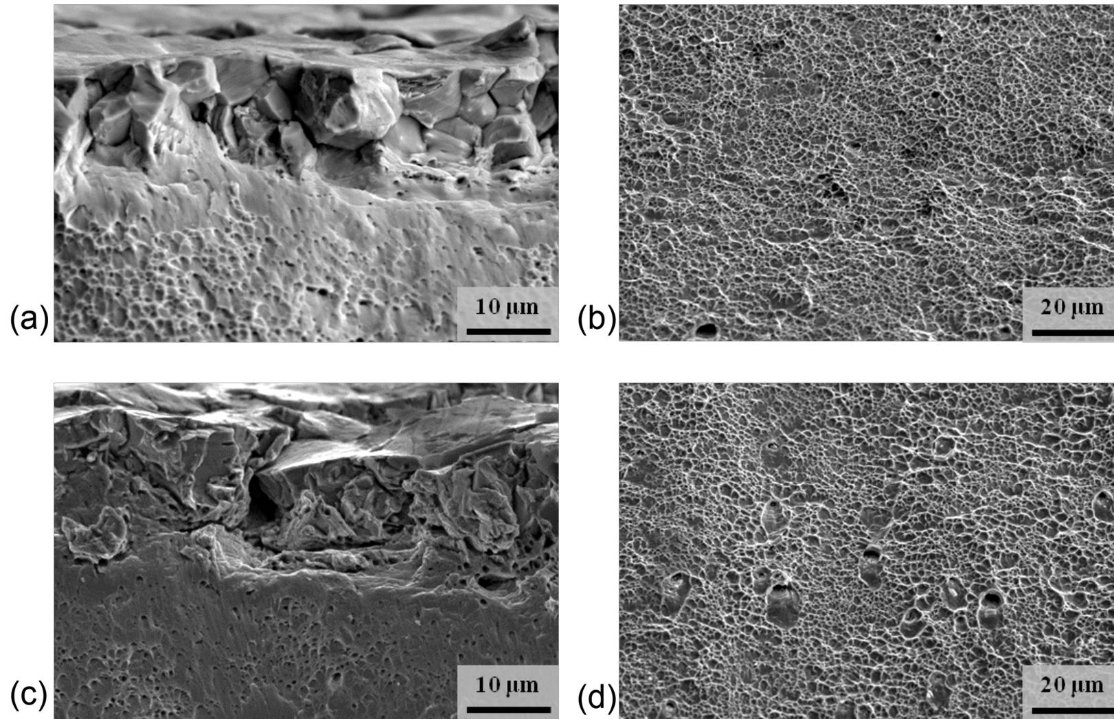
Figure 3 Fracture surfaces of the hydrogen charged (a,b) TW1 and (c,d) TW2 alloys after tensile test: (a), (c) represent fractography near the specimen surface. (b), (d) are magnified view of specimen centre.
