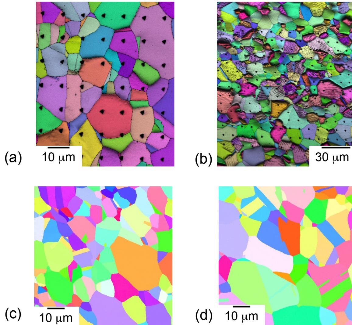
Figure 1. EBSD band contrast map of TW1 alloy after indenting (a) 7×7 arrays for hydrogen uncharged and (b) 15×15 arrays for hydrogen charged condition. Typical EBSD mapping of annealed (c) TW1 and (d) TW2 alloys.
