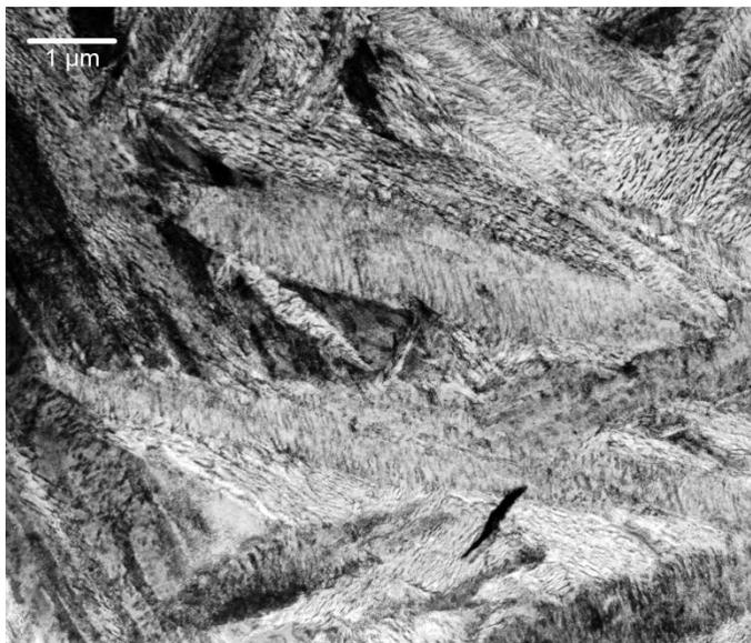
Figure 10: Lower bainitic microstructure of 52100 steel, isothermal holding at 230°C for 10 h (Vetters *et al.* 2006).
