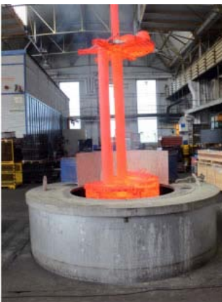
Fig. 1: Huge samples of the steel described here undergoing heat-treatment (in this case austenitisation). For more details, see Nanostructured bainite, Proceedings of the Royal Society of London - A, Vol. 466, 2010, 3–18, and The first bulk nanostructured metal, Science and Technology of Advanced Materials 14 (2013) 014202. The first bulk nanostructured metal These and other articles can be downloaded from www.msm.cam.ac.uk/phase-trans/2010/nano.html
