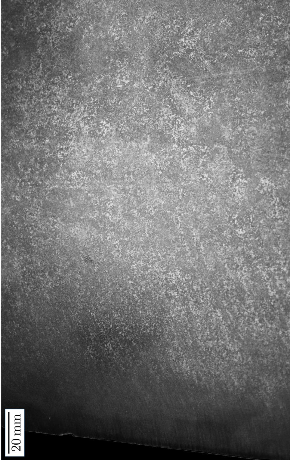
**Figure 8.21:** Area of Face A labelled (ii). Columnar dendritic formations can be seen protruding in from the left-hand edge at an upwards angle to the horizontal. They appear to stop after growing  $\approx 12$  cm into the ingot.
