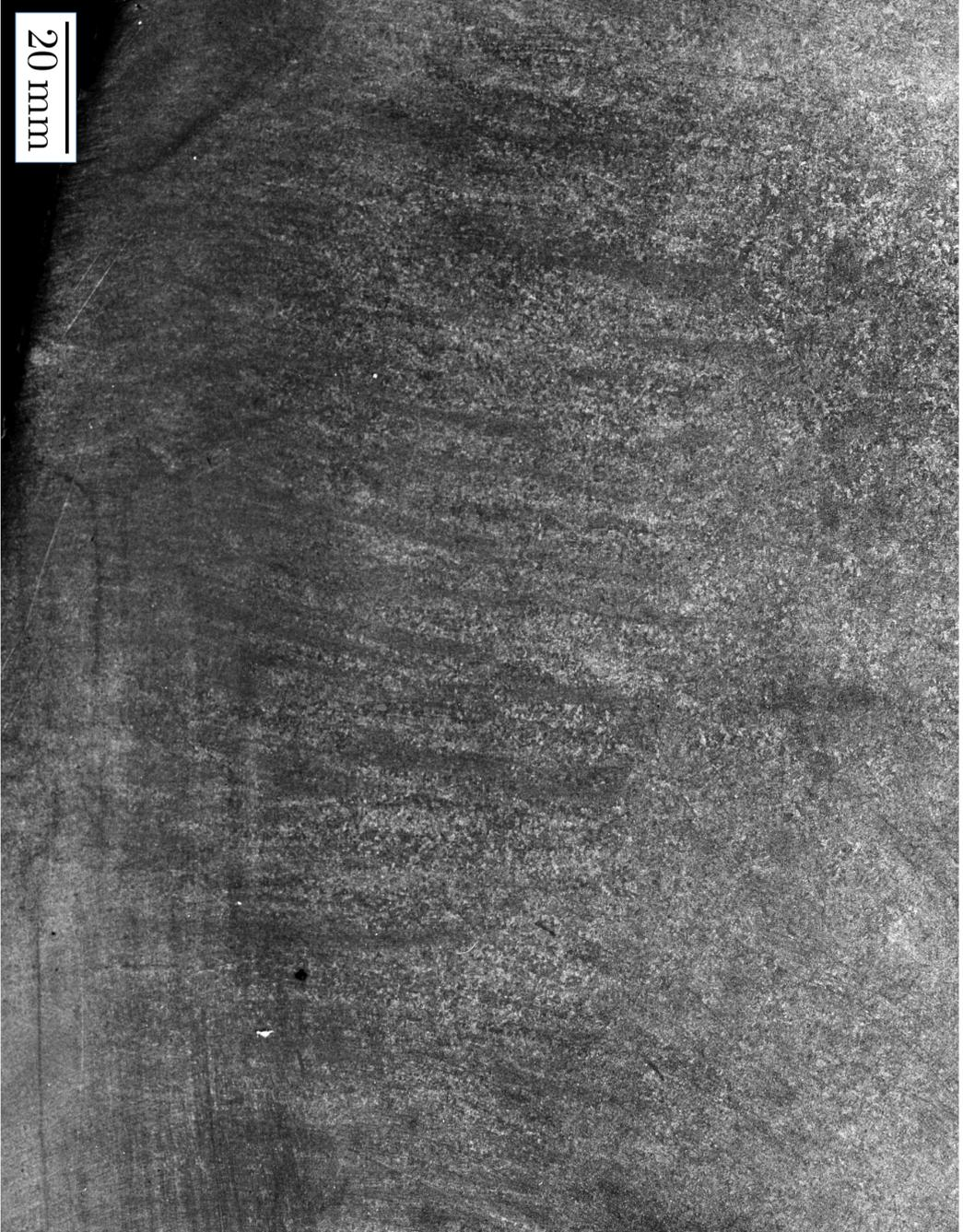
**Figure 8.22:** Area of Face A labelled (iii), found at the base of the ingot. Columnar dendritic formations appear to have grown from the bottom edge for  $\approx 12$  cm.
