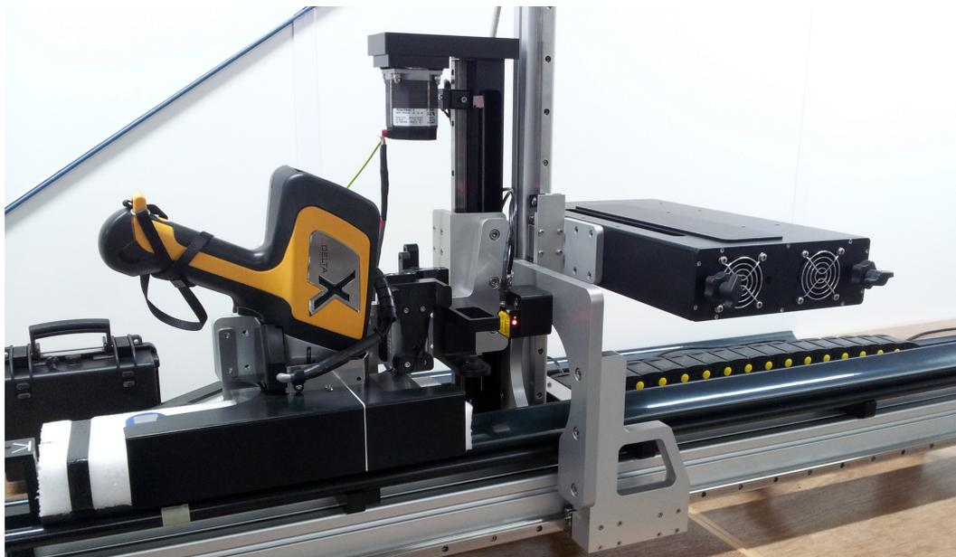
**Figure 7.1:** The automated XRF apparatus. A standard hand-held XRF is mounted on a robotic gantry system with laser-guided movement.
