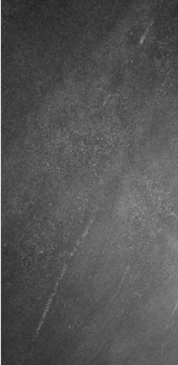
**Figure 8.29:** A-segregate strings, present towards the bottom of the ingot. The channels were  $\approx 5$  mm in diameter.
