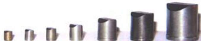
Figure 15: Fragment Simulator Projectiles, defined in MII-P-46593A, made of 40 NiCrMo 84 (1.6562), HRC 30. From 0.237 g / 3.25 mm to 13.4 g / 12.9 mm
