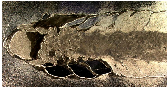
Figure 28: Penetration of a W sinter rod in P900 target. V_p = 1700 m/s, \sigma_{rod} = 1800 MPa, \sigma_{target} = 1200 MPa
