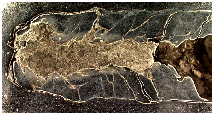
Figure 29: Penetration of a W sinter rod in P900 target. V_p = 1700 m/s, \sigma_{rod} = 1800 MPa, \sigma_{target} = 2000 MPa
