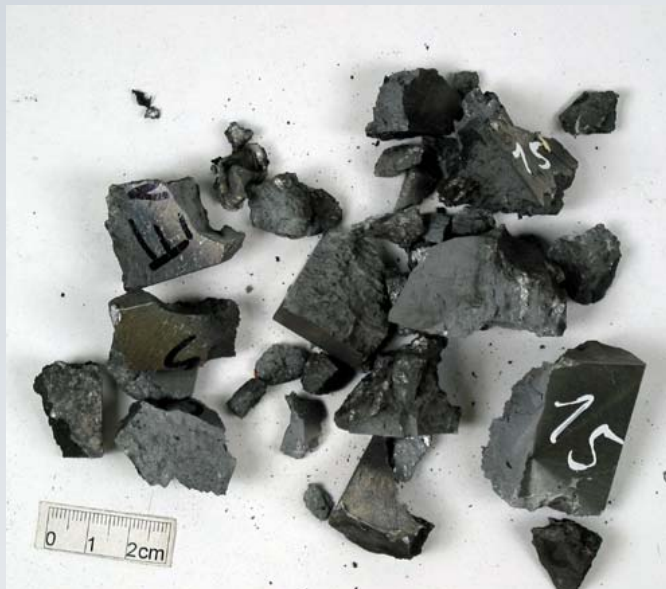
AlSi7Mg reinforced by SiC- particles of size F1200
