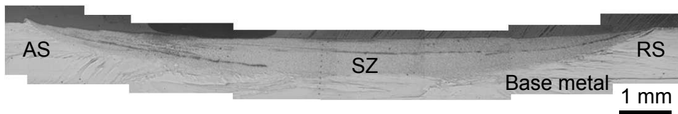
Fig. 3 Cross-section of Fe-7Al alloy after FSP with SiC addition.
