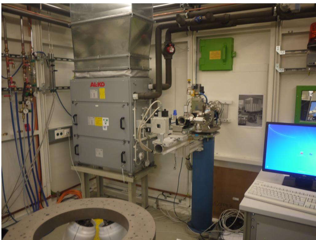
**Figure 3.4:** DESY P07 beam line showing beam collimator.
