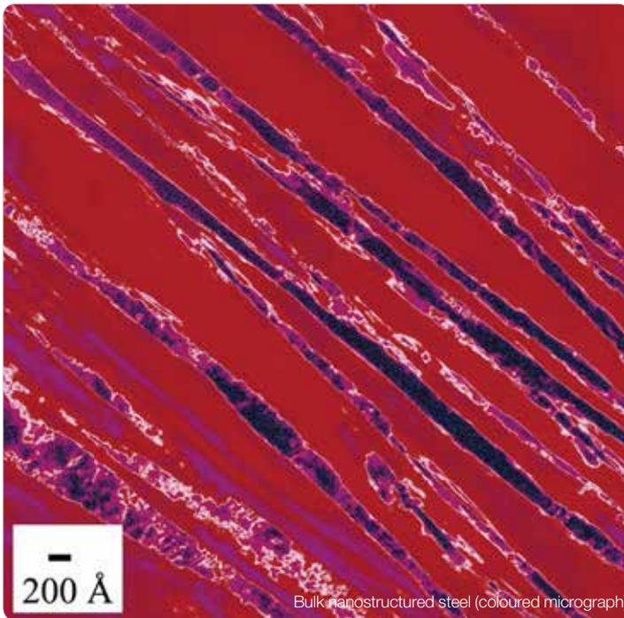
Bulk nanostructured steel (coloured micrograph)
