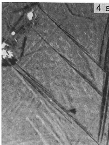
Fig. 6.14 Photoemission electron microscope observations on the growth of individual sub-units in a bainite sheaf (Bhadeshia, 1984). The pictures are taken at 1 s intervals during transformation at 380 Centigrade in a Fe-0.43C-2.02Si-3Mn wt% alloy. The micrograph at 0 s is fully austenitic, the relief being a residue from a previous experiment.
