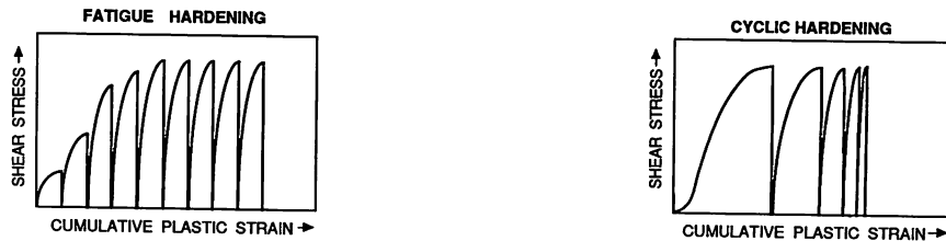
Fig. 12.13 Schematic illustration of constant plastic strain and constant stress fatigue tests (after Kettunen and Kocks, 1967).
