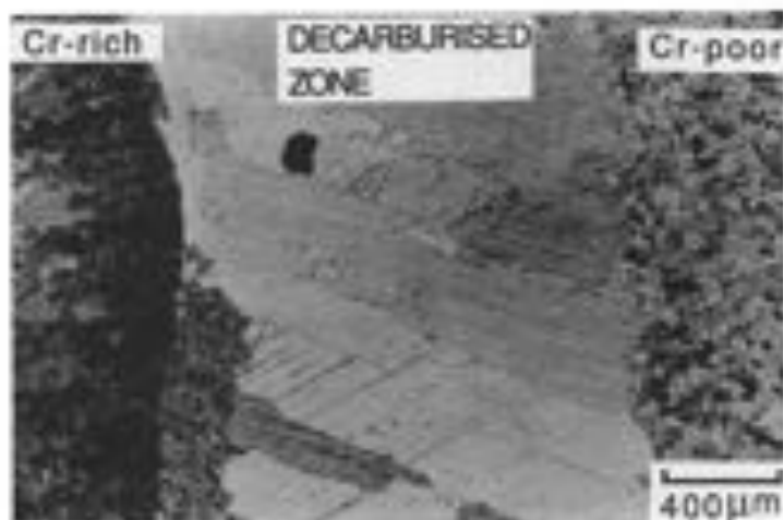
Fig. 12.19 Optical micrograph of a junction between mild steel and a 2.25Cr-1Mo alloy, showing the development of a decarburised zone in the mild steel side of the joint after tempering (After Race, 1990).
