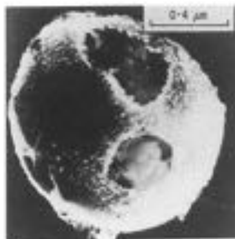
Fig. 10.2 Scanning transmission electron micrograph of a nonmetallic inclusion in a steel weld metal. The inclusion surface is very irregular, and it features many planes. (Barrille, 1992).
