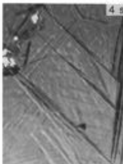
Fig. 6.14 Transmission electron microscope observations on the growth of individual sub-units in a bainitic steel (Bhadeshia, 1984). The pictures are taken at 1 s intervals during transformation at 380 Centigrade in a Fe-0.43C-2.025Si-3Mn wt% alloy. The micrograph at 0 s is fully austenitic, the relief being a residue from a previous experiment.
