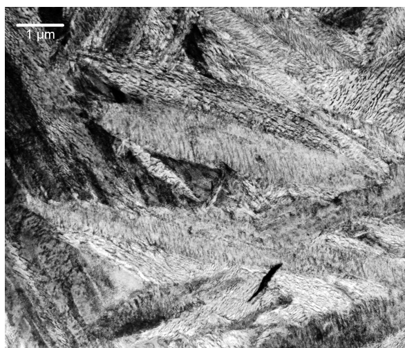
Figure 13.61 Lower bainite generated by isothermal transformation of 52100 steel at 230 °C for 10 h (Vetters et al., 2006). Micrograph kindly provided by J. Dong and H.-W. Zoch.
