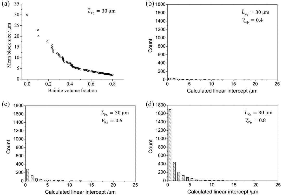
Figure 4: Calculated result for  $\bar{L}_{\gamma_0} = 30 \mu\text{m}$ . (a) Mean blocky austenite size as a function of bainite volume fraction, (b) Retained austenite size distribution for  $V_{\alpha_b} = 0.4$ , (c) Retained austenite size distribution for  $V_{\alpha_b} = 0.6$ , (d) Retained austenite size distribution for  $V_{\alpha_b} = 0.8$ .
