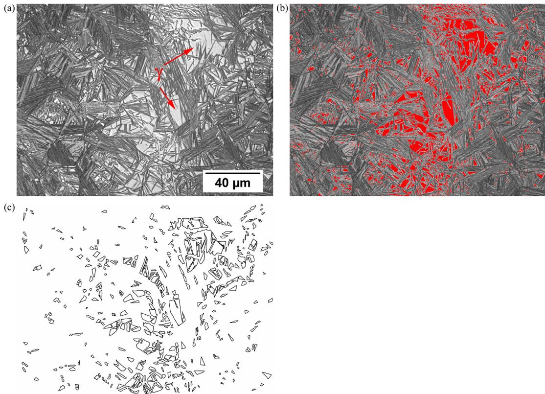
Figure 7: (a) Optical micrograph of steel B transformed at 250 °C for 48 h used for blocky retained austenite size distribution measurement. (b) Selection of blocky retained austenite by ImageJ threshold method. (c) Retained austenite blocks by manual drawing.
