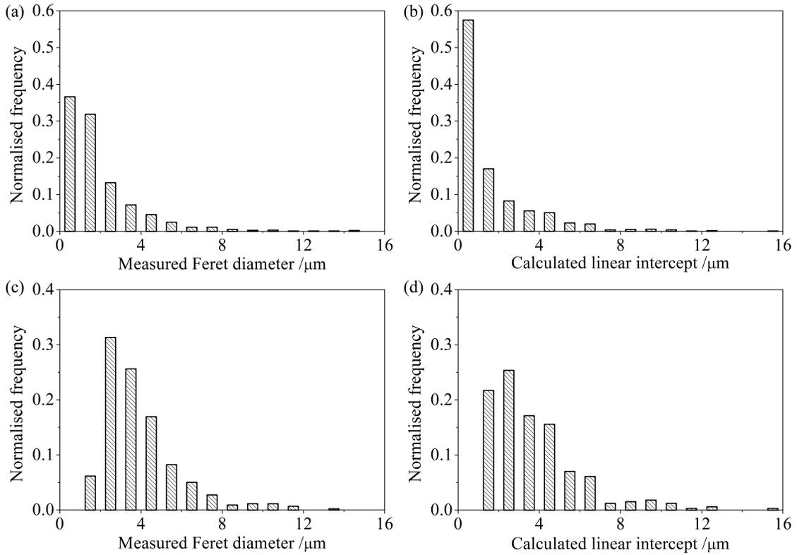
Figure 8: Retained austenite size distribution of steel A isothermally transformed 250 °C for 48 h. (a) Measured using threshold and particle analysis technique in ImageJ software. (b) Calculated with  $\bar{L} = 24 \mu\text{m}$  and  $V_{\alpha_B} = 0.66$ . (c) Measured by manual drawing retained austenite blocks on micrograph. (d) Calculated with compartments smaller than the minimum value of manually measured ones excluded.
