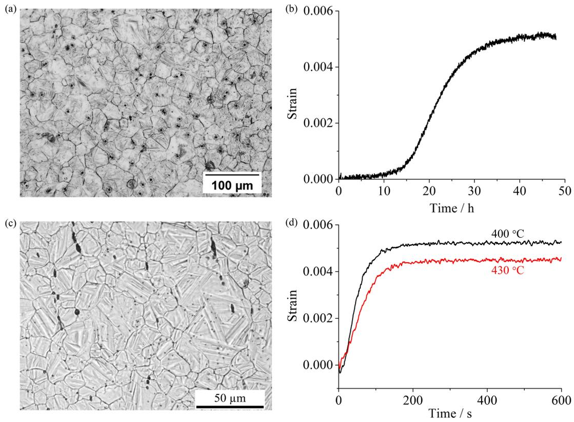
Figure 6: (a) Optical micrograph showing prior austenite grain boundaries of steel A austenitised at 1000 °C for 10 min. (b) Strain as a function of time of steel A isothermally transformed at 250 °C for 48 h. (c) Optical micrograph showing prior austenite grain boundaries of steel B austenitised at 950 °C for 10 min. (d) Strain as a function of time of steel B isothermally transformed at 400 and 430 °C for 1 h.
