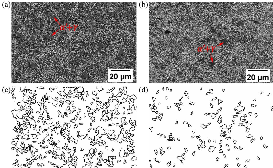
Figure 9: Measurement of  $\alpha' + \gamma$  constituent. (a) Secondary electron image of steel B transformed at 430 °C for 1 h, (b) 400 °C for 1 h. (c)  $\alpha' + \gamma$  island by manual drawing for (a). (d)  $\alpha' + \gamma$  island by manual drawing for (b).
