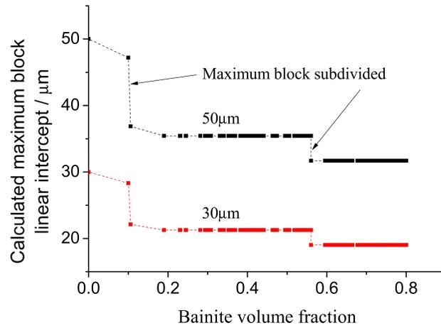
Figure 3: Calculated maximum retained austenite size as a function of bainite volume fraction for  $\bar{L}_{\gamma_0} = 50$  and 30  $\mu\text{m}$ .
