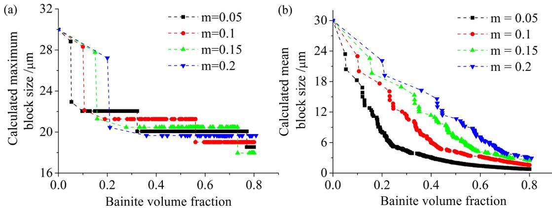
Figure 2: (a) Effect of  $m$  on the maximum compartment size. (b) Effect of  $m$  on the average block size.
