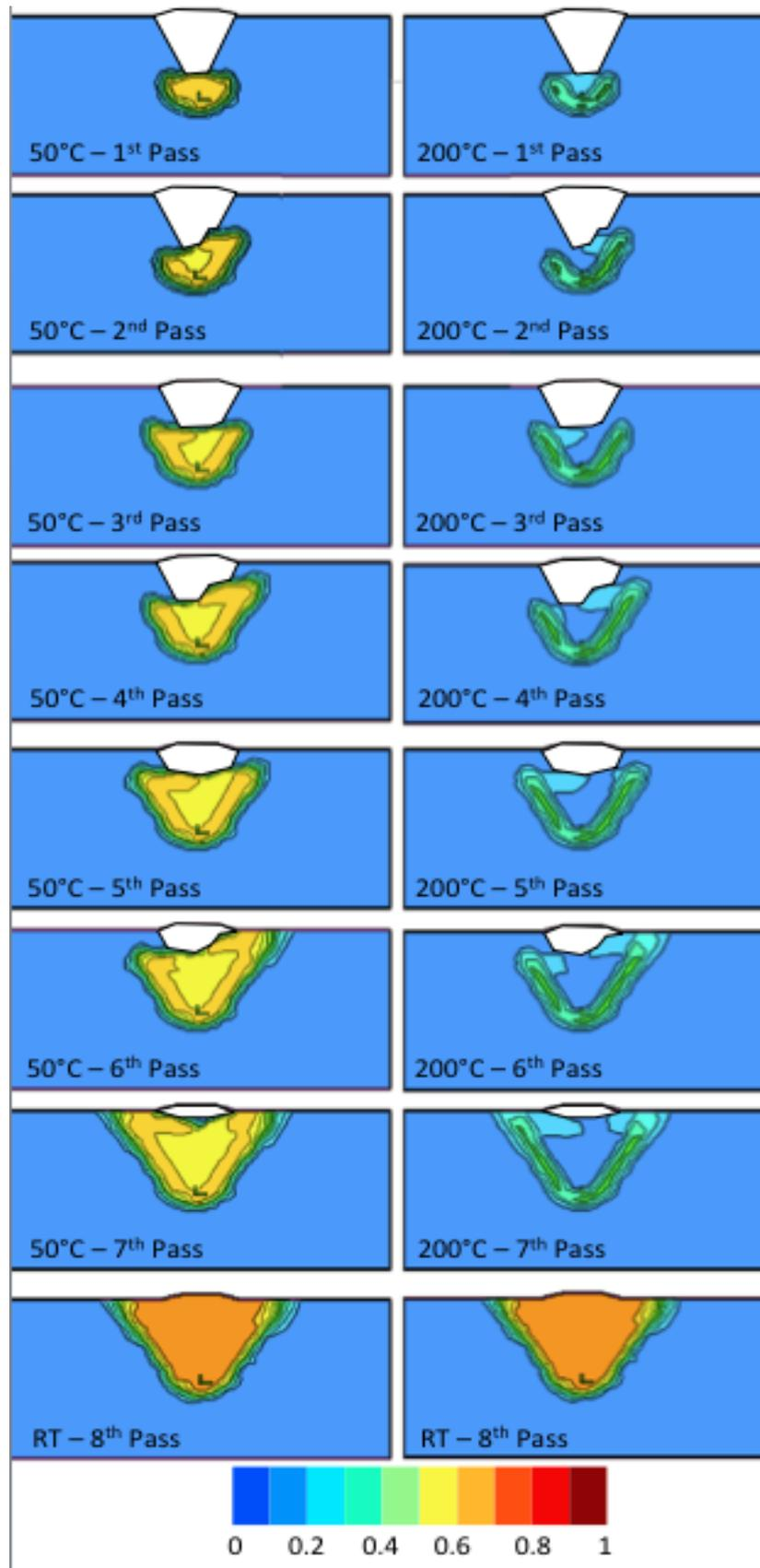
Figure 8: The predicted martensite fraction for after the laying down of each pass for interpass hold temperatures of 50°C (left) and 200°C (right) . After the 8<sup>th</sup> pass the plate has been allowed to cool to room temperature.
