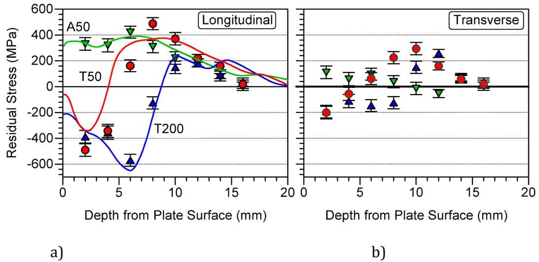
Figure 5: a) Longitudinal and b) transverse residual stress profiles with depth through the thickness of the plates at the weld-centreline. The markers denote neutron diffraction measurements while in (a) the corresponding continuous lines denote the contour method results for the same plate.
