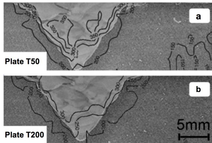
Figure 3: a) and b) weld microstructures and microhardness maps (in HV2) for the plate T50 (50°C interpass temperature) and plate T200 (200°C interpass temperature) welds respectively
