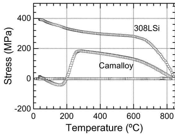
Figure 1: a) Stress recorded during constrained cooling (Sato test) of the two filler metals used in this study [12]
