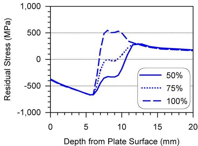
Figure 11: Effect of final austenite fraction on the predicted stress when the interpass temperature is kept at 50°C.
