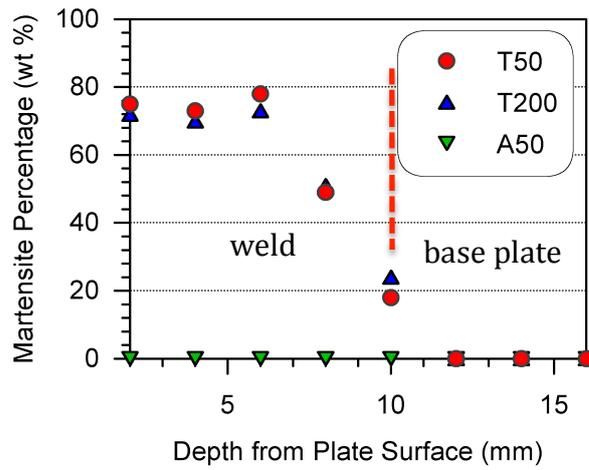
Figure 4: Variation in martensite fraction from top surface to weld root as determined by neutron diffraction.
