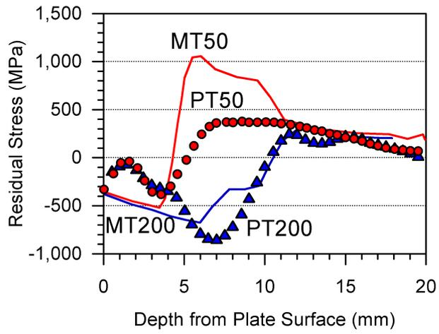
Figure 10: Predicted longitudinal residual stresses (continuous lines) plotted alongside the contour method measurements for similar conditions (modelled data denoted M and contour data denoted P)
