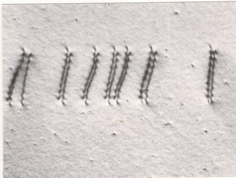
Figure 5.17 Paired dislocations in quenched Ni-8.7at.%Al-2.5at.%Ti.
