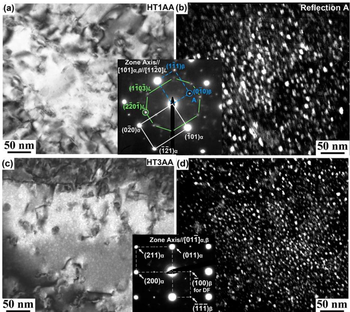
Figure 15 (a) TEM BF micrograph after HT1AA with SADP in insertion showing ferrite,  $\beta$ -NiAl superlattice and Laves phase reflections; (b) DF image of the same area of (a) using the  $\beta$ -NiAl  $(0\bar{1}0)_\beta$  superlattice reflection labelled as A in the SADP. (c) BF micrograph after HT3AA with SADP in insertion, (d) DF image of the same area of (c) using the  $\beta$ -NiAl  $(\bar{1}10)_\beta$  superlattice reflection.
