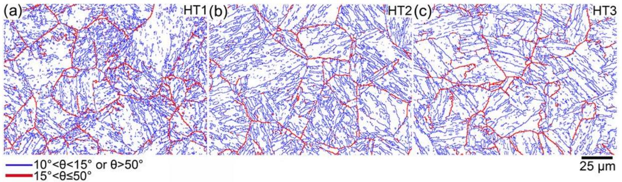
Figure 8 Microstructures of the martensitic matrix as disorientation boundaries maps in the materials subjected to (a) HT1, (b) HT2 and (c) HT3.
