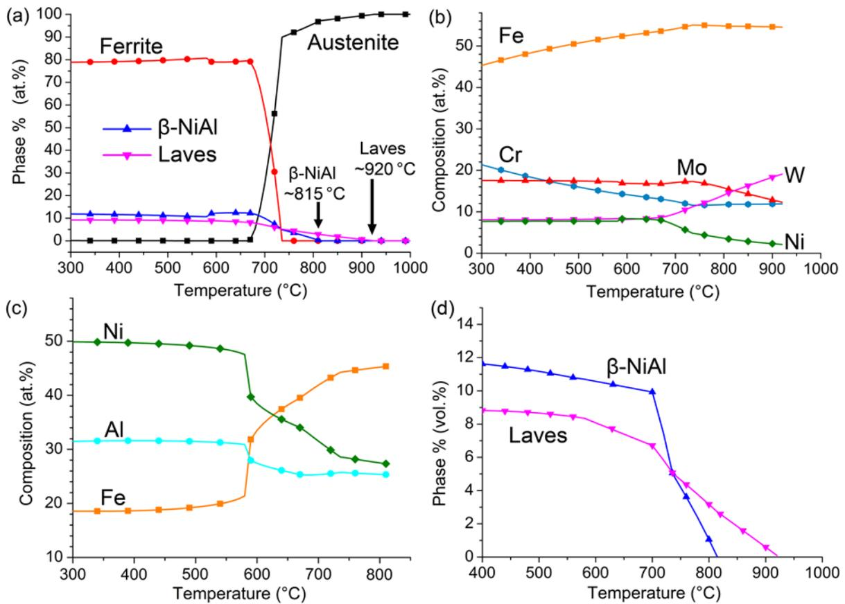
Figure 1 Equilibrium thermodynamics calculation using MatCalc: (a) all phase in at.%, (b) composition of the Laves phase and (c) composition of the  $\beta$ -NiAl as functions of temperature; (d) the calculated volume percentages of Laves phase and  $\beta$ -NiAl.
