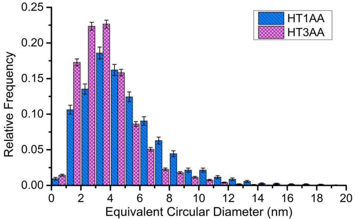
Figure 17 Histograms showing the size distributions of the  $\beta$ -NiAl phase precipitates after heat treatment HT1AA and HT3AA.
