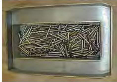
Figure 7: Test load with 5 kg net-weight of plungers (d = 8 mm, l = 54 mm)
