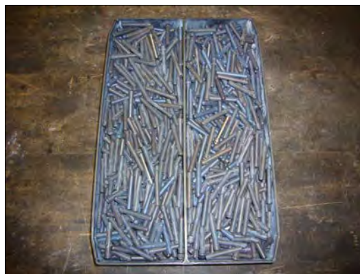
Figure 9: Test load with 23 kg net-weight of plungers (d = 8 mm, l = 54 mm)
