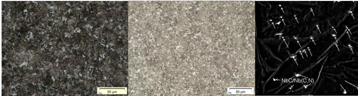
Figure 4: Microstructure investigations: LOM 18CrNiMo7-6 (left); LOM 18CrNiMoNb7-6 (middle); TEM-dark field image with Nb(C,N)-precipitates in 18CrNiMoNb7-6; 10000x magnification (right); all samples blank-hardened
