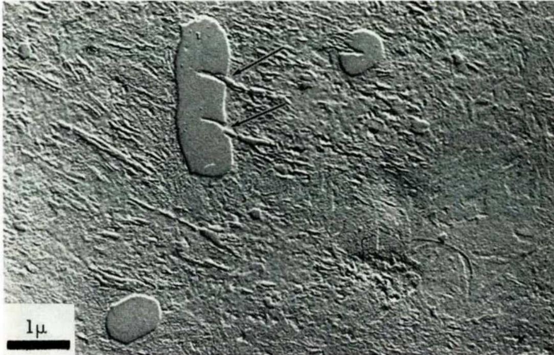
**Figure 28.** SAE 52100 steel ball bearing inner race. Transverse section showing intrusions (arrows) and extrusions along edge of undissolved iron carbide particle. Etched in picral [31].
