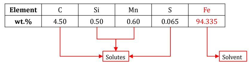
**Note**: the main difference between hot metal and liquid steel is the content of carbon.
