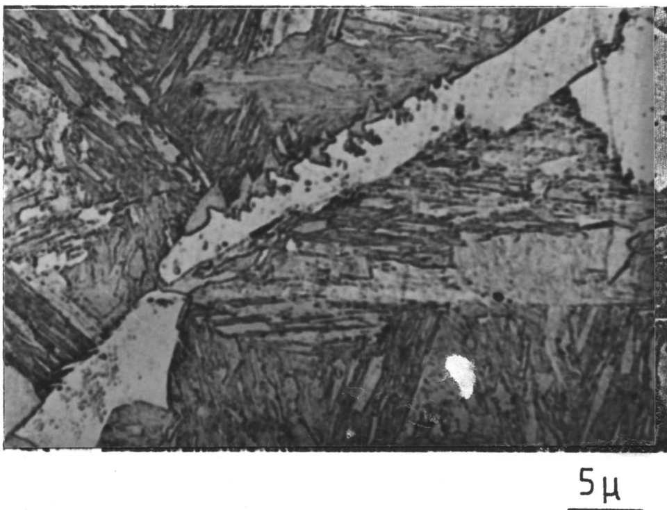
Figure 8.28: Showing evidence of interface pinning. (610°C/20 min).
