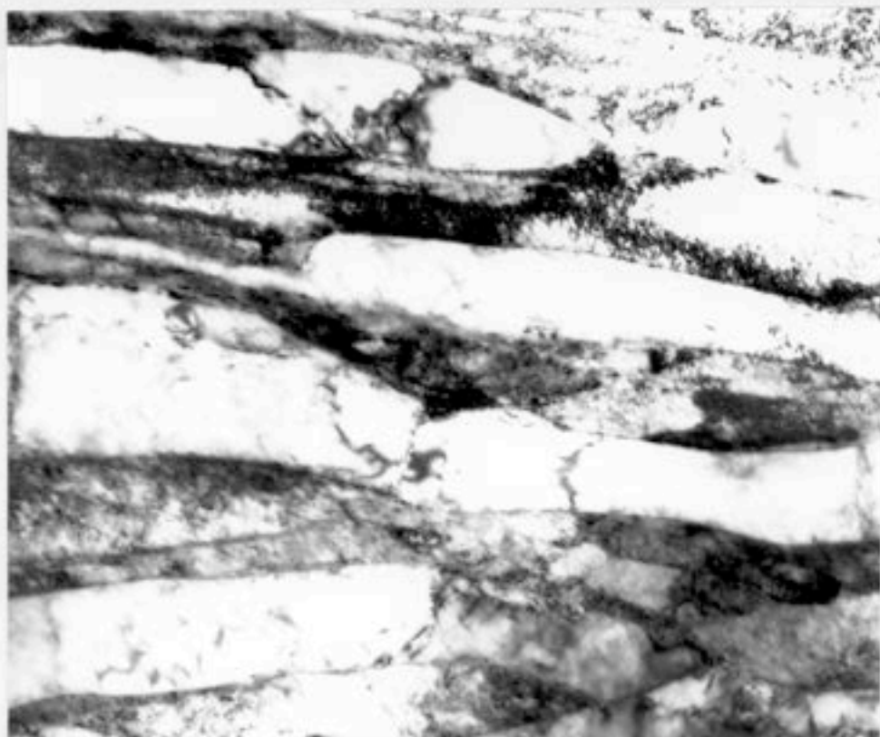
Figure VII.14c - 10 mins @ 950°C → 2 hrs @ 350°C → 2 hrs @ 720°C → quenched by helium gas.
