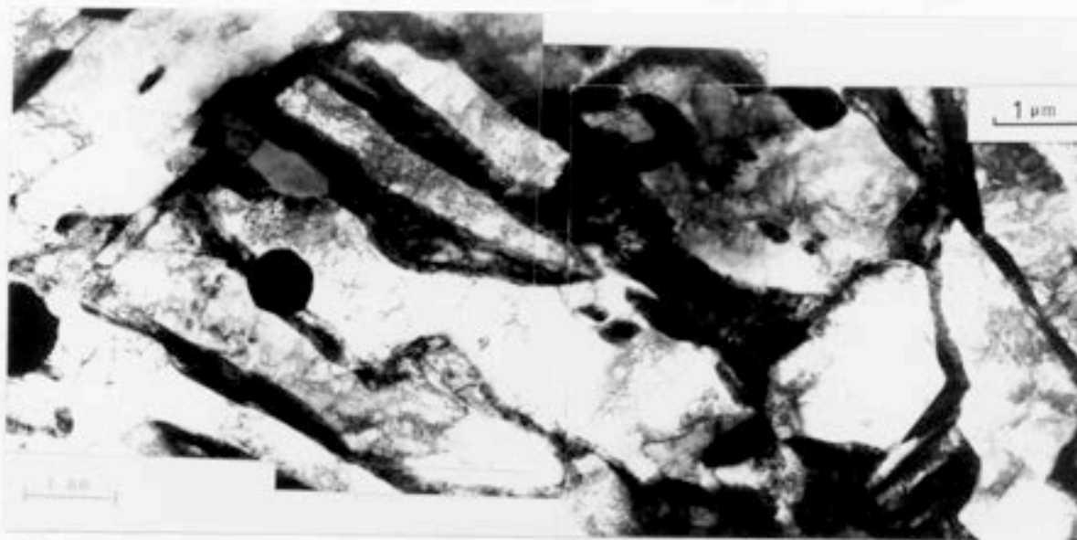
Figure IV.7(b) - Reaustenitisation at 700°C for 10 minutes from starting microstructure \alpha_a + \gamma .
