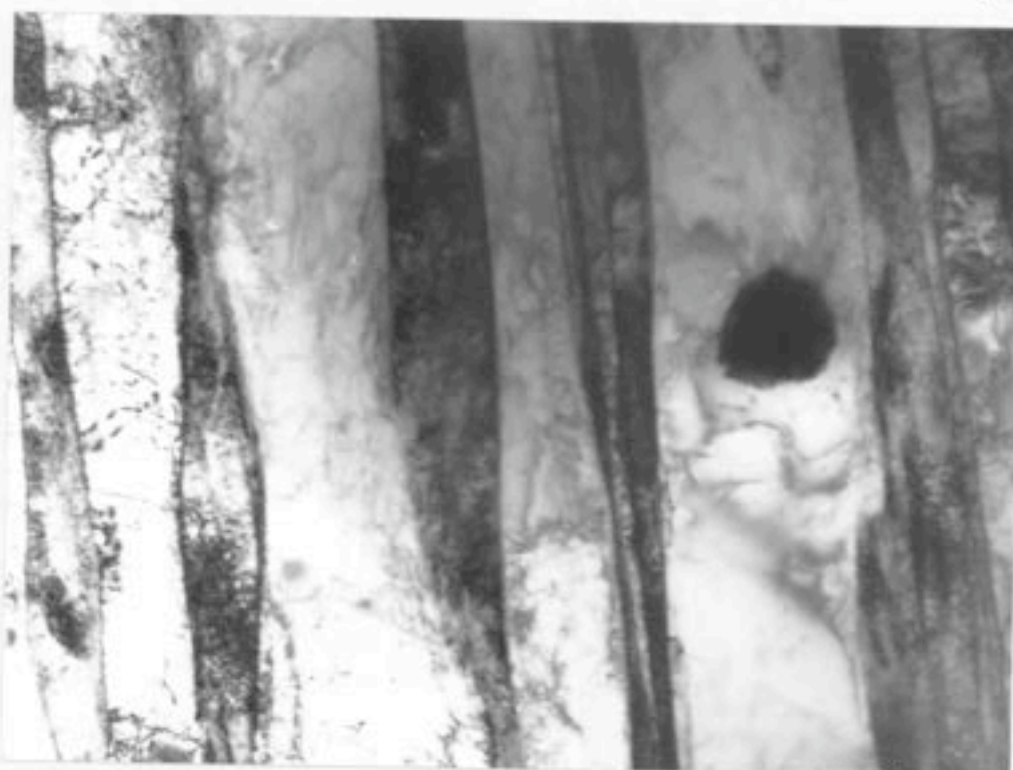
Figure IV.6(b) - Reaustenitisation at 700°C for 2 hours from starting microstructure \alpha_b + \gamma .
