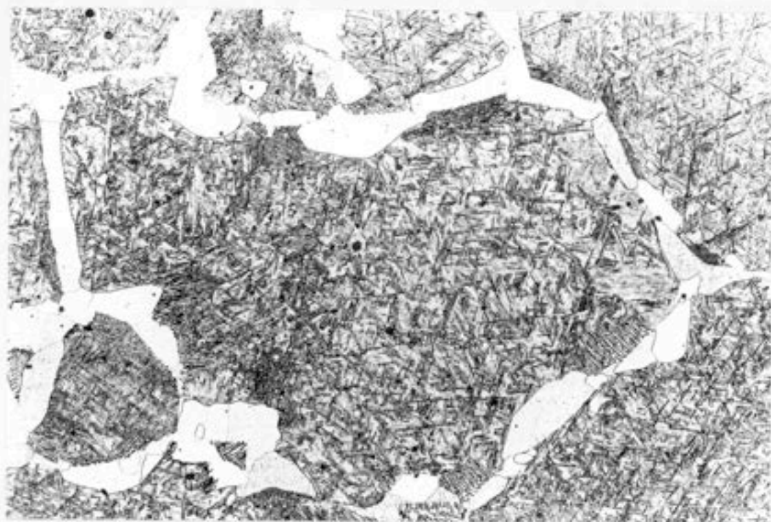
Figure VIII.8(c) - 10 mins @ 1200°C → 2 hrs @ 720°C → quenched by helium gas. 50μm
