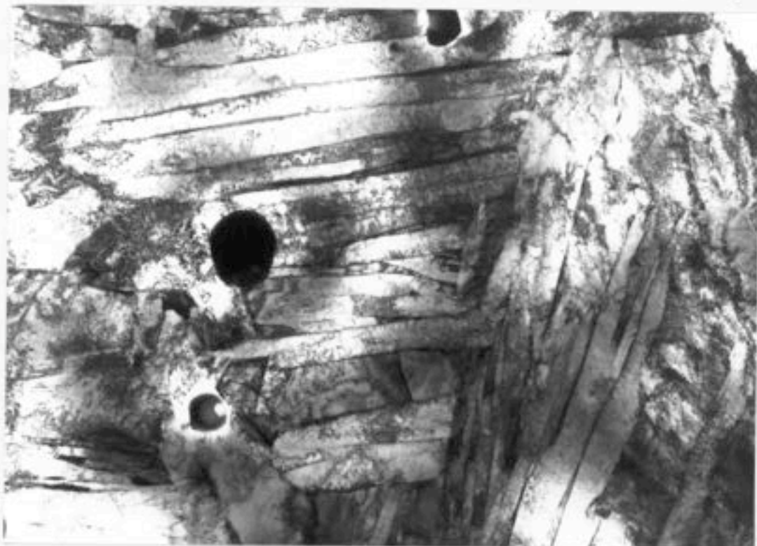
Figure IV.6(f) - Reaustenitisation at 760°C for 2 hours from starting microstructure \alpha_b + \gamma .
