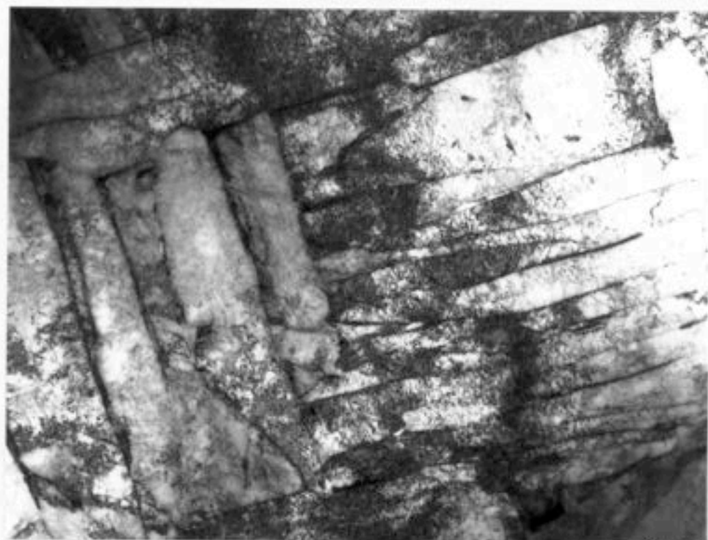
Figure IV.7(e) - Reaustenitisation at 760°C for 2 hours from starting microstructure \alpha_a + \gamma .
