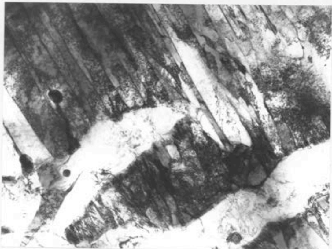
Figure IV.6(e) - Reaustenitisation at 750°C for 2 hours from starting microstructure \alpha_b + \gamma .
