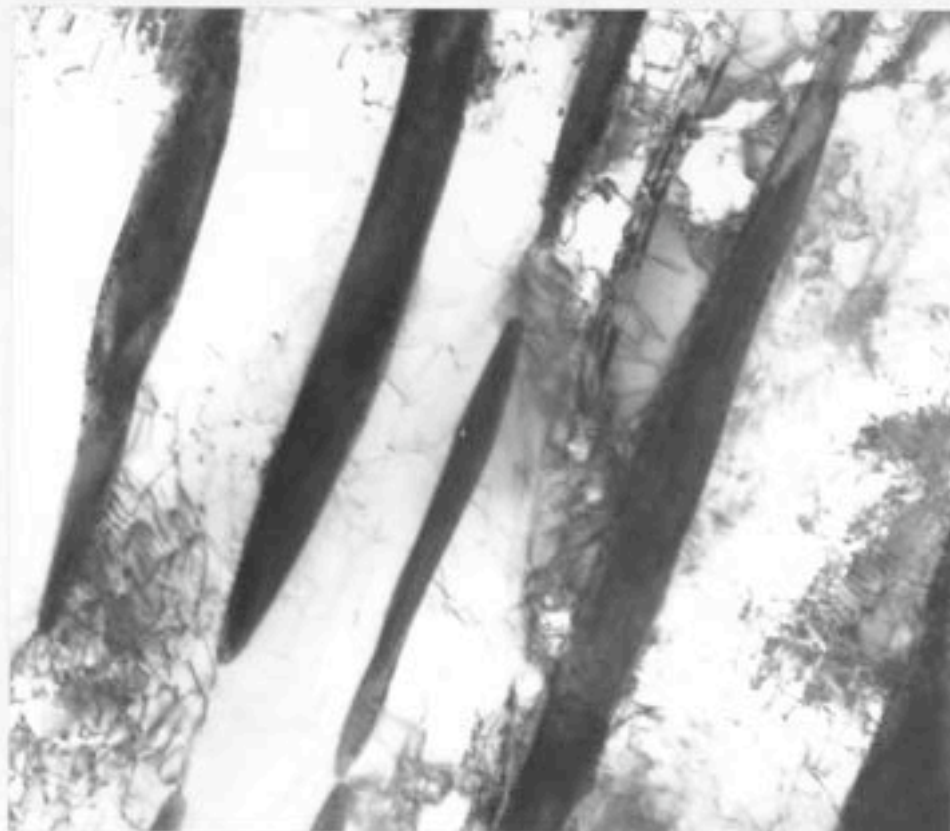
Figure IV.6(a) - Reaustenitisation at 680°C for 2 hours from starting microstructure \alpha_b + \gamma .
