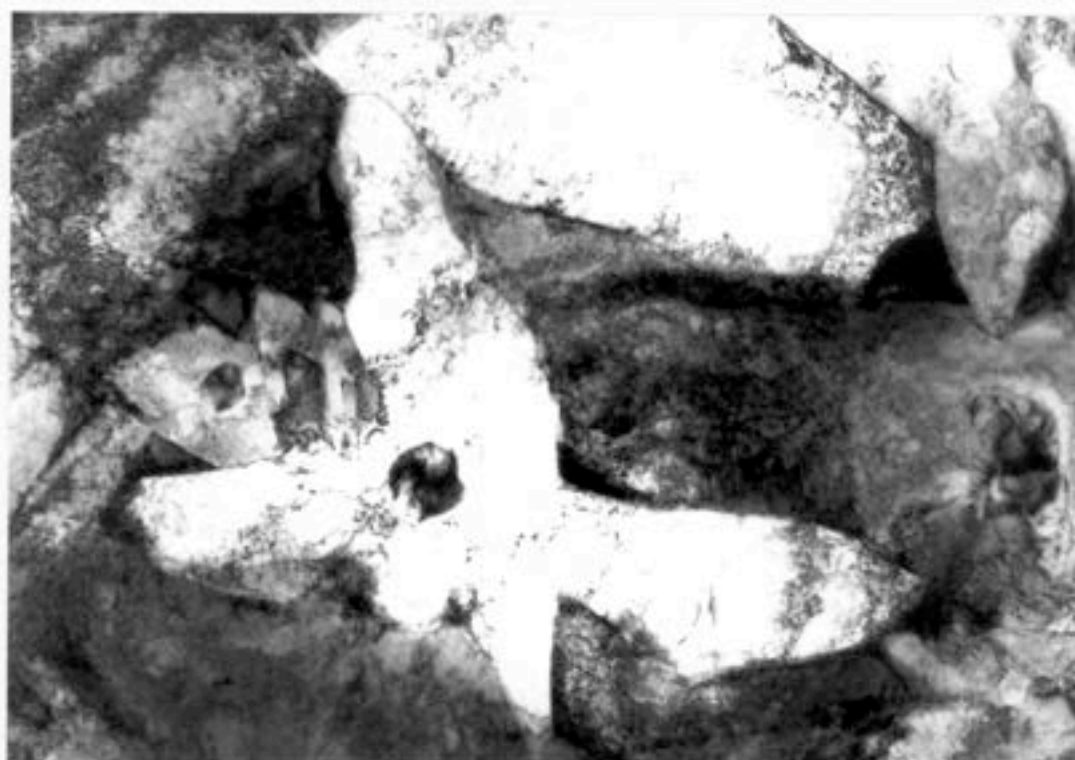
Figure II.7(d) - Electron micrograph shows that several acicular ferrite plates grow from one inclusion in fusion zone of weld metal WD2.
