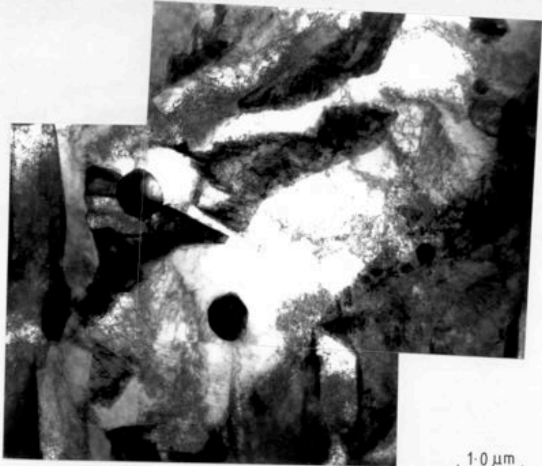
Figure IV.7(c) - Reaustenitisation at 720°C for 2 hours from starting microstructure \alpha_a + \gamma .
