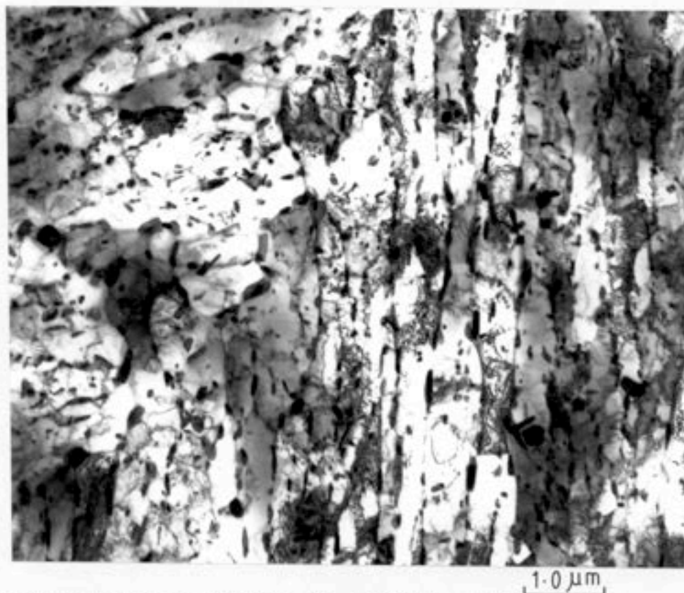
Figure VII.17 - 10 mins @ 950°C → 2 hrs @ 350°C → 42.7 hrs @ 600°C.
