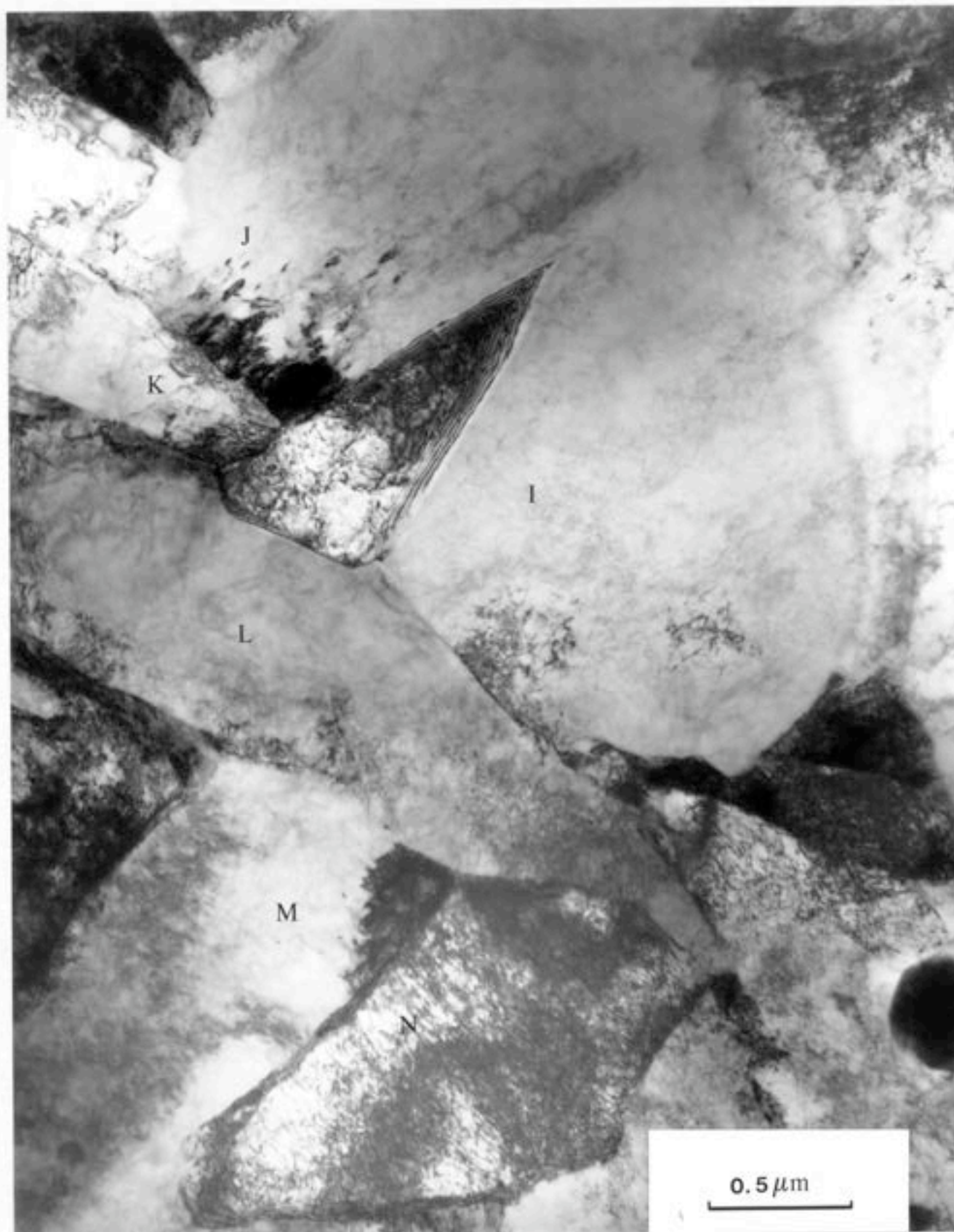
Figure VI.6 - Electron micrograph shows six acicular ferrite plates designated I,J,K,L,M and N, which are in intimate contact.
