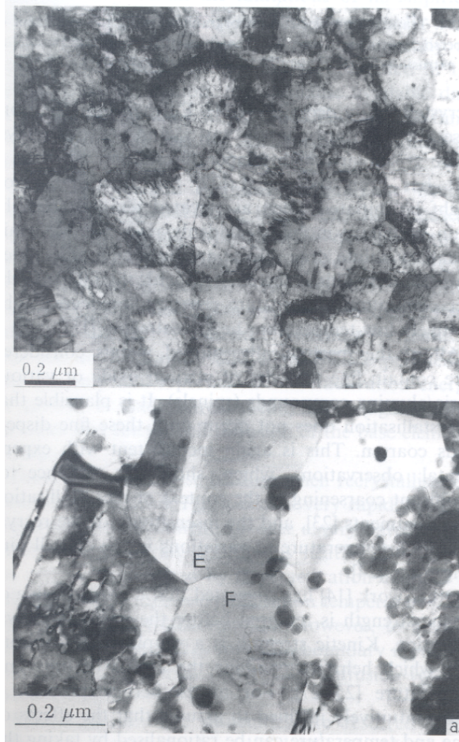
Fig. 2: Transmission electron micrographs showing the sub-micron grain structure of mechanically alloyed and consolidated alloys. (a) Iron-base MA956. (b) Nickel-base MA6000; electron diffraction confirms that there are large misorientations across grains such as E and F . The grains in both cases do not represent low-misorientation cells of the type common in ordinary deformation. Both micrographs are sections normal to the extrusion direction. The appearance of MA6000 microstructure is independent of the plane of section, but the microstructure of MA956 is cold-deformed and hence the grains are elongated along the extrusion direction.
