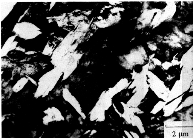
Fig. 5—A transmission electron micrograph illustrating the morphology of acicular ferrite in a steel weld deposit.
