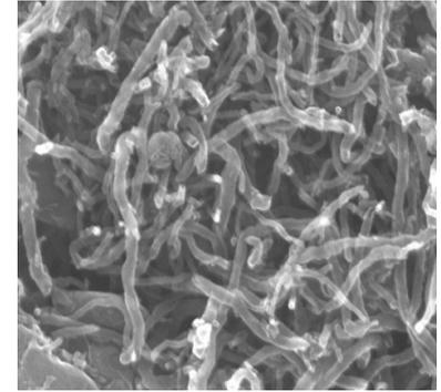
In recent years, nanostructured carbon forms, such as fullerenes and carbon nanotubes (MWCNT) become more often used for modifying and preparation of carbon composite materials based on metals, alloys, polymers, and ceramics. Production processes used for these materials exhibit a great variety. More frequently, the modification of materials by nanostructured carbon forms is performed by high-energy milling and hot pressing.
