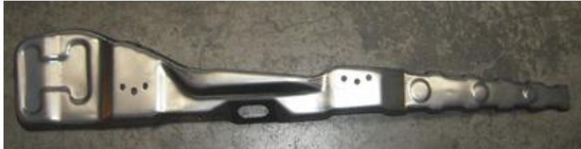
B-pillar Reinforcement L/R Gauge: 2.0 mm
