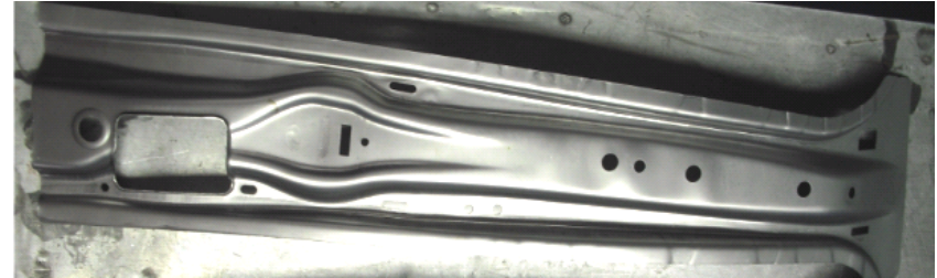
B-Pillar Inner Gauge: 1.2 mm
