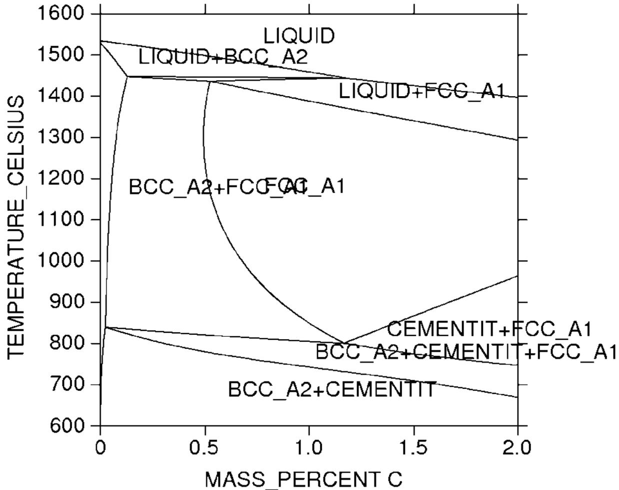
Moving eutectoid carbon from ~0.5 to ~ 1.2 wt%
