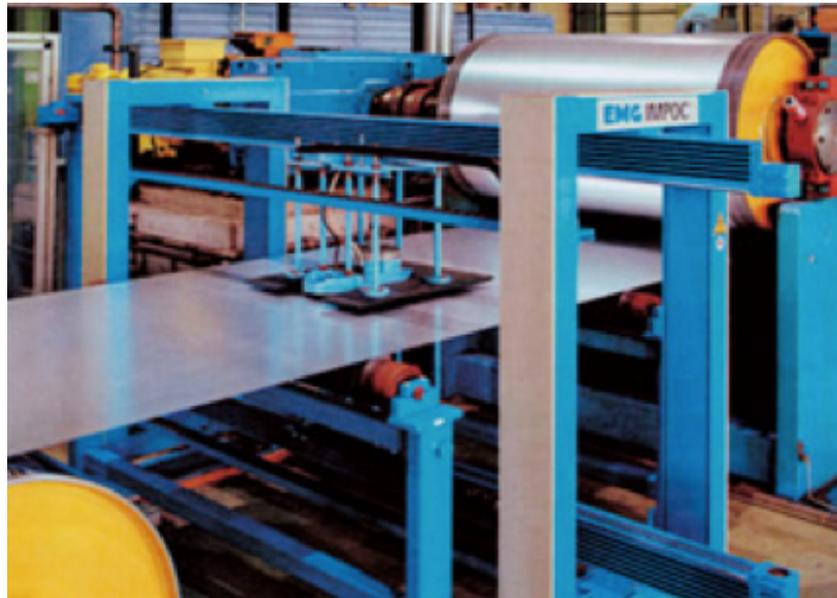
IMPOC system for cold rolled strip product for tensile strength prediction
