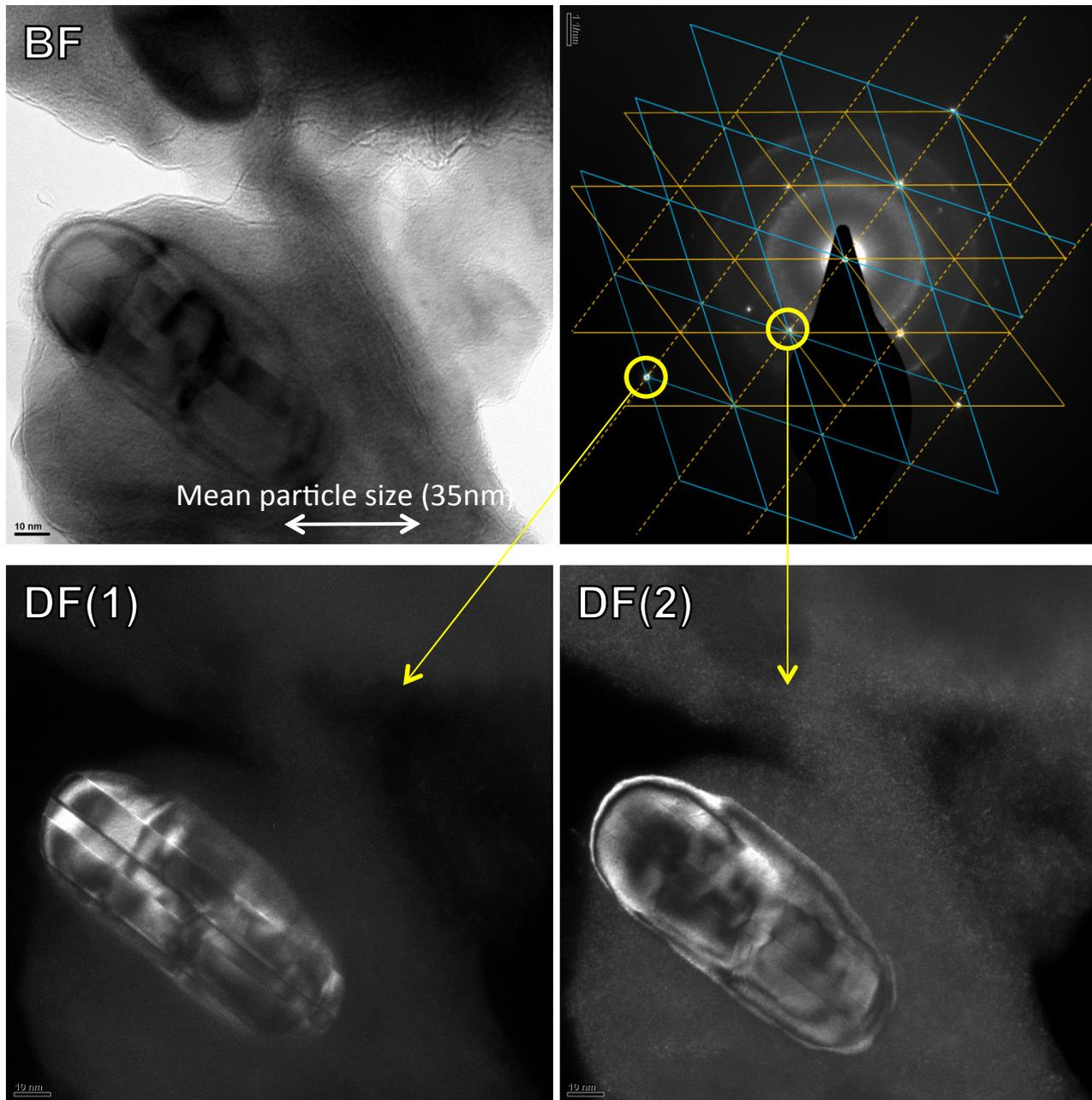
**5% cold-rolled specimen** beam//[111]<sub>Fe</sub>
