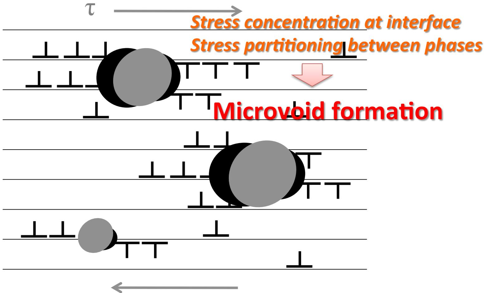
Ductile fracture is enhanced
