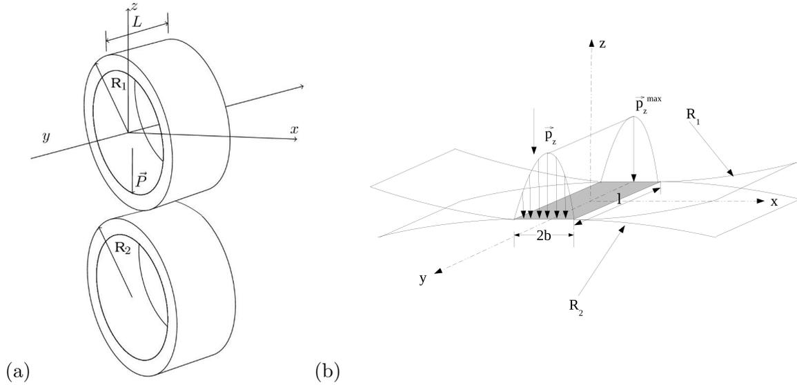
Figure 1: Schematic of the (a) twin-disc set up, (b) stress distribution over the Hertzian contact.
