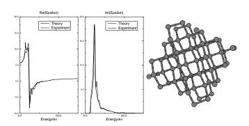
The complex dielectric function for diamond was calculated with a 0.5ev Gaussian smearing and a 0.7ev Scissor operator applied to the conduction bands.
